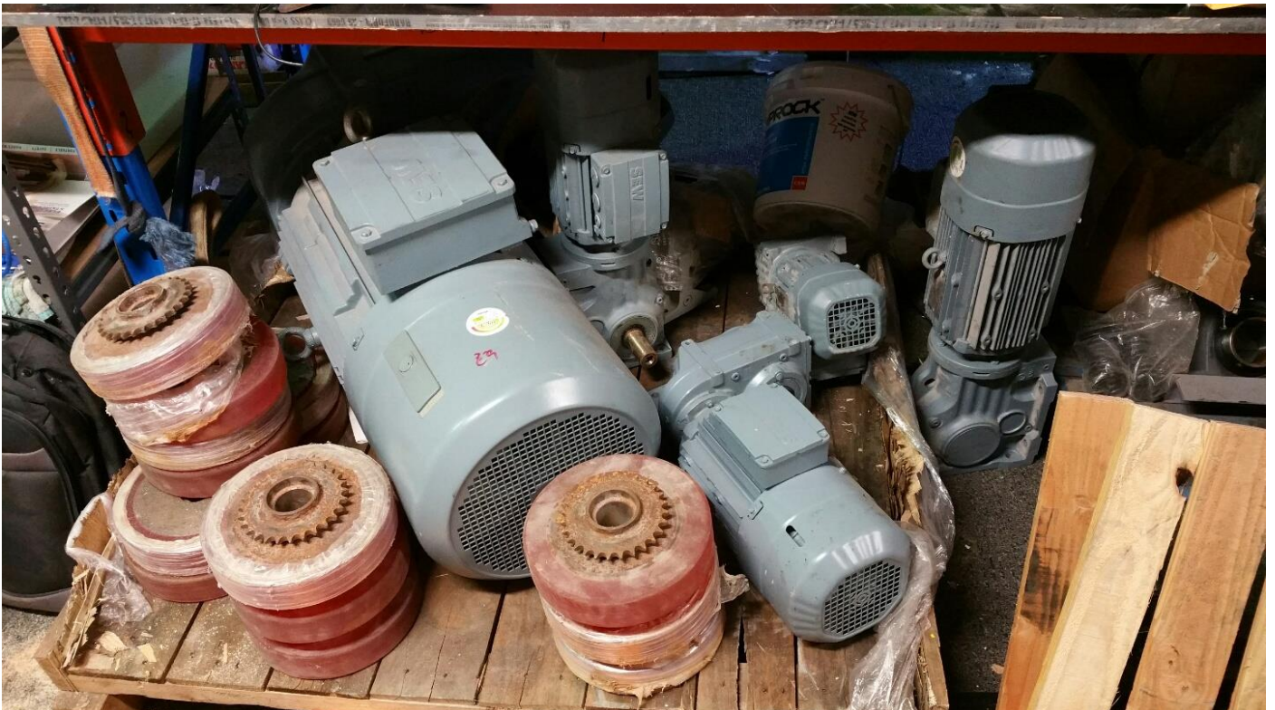
(Figure 6; 45 Maxwell St, Newfarm. Main lifting motoring and driving mechanism)
